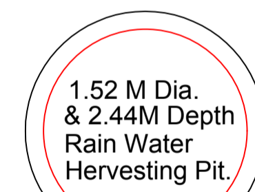
PLAN OF RAIN WATER HARVESTING
