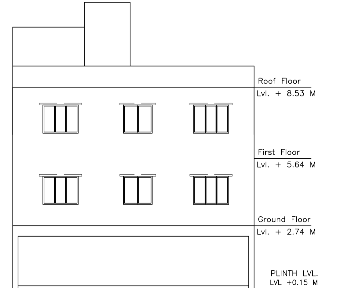
FRONT ELEVATION SCALE - 1:100
