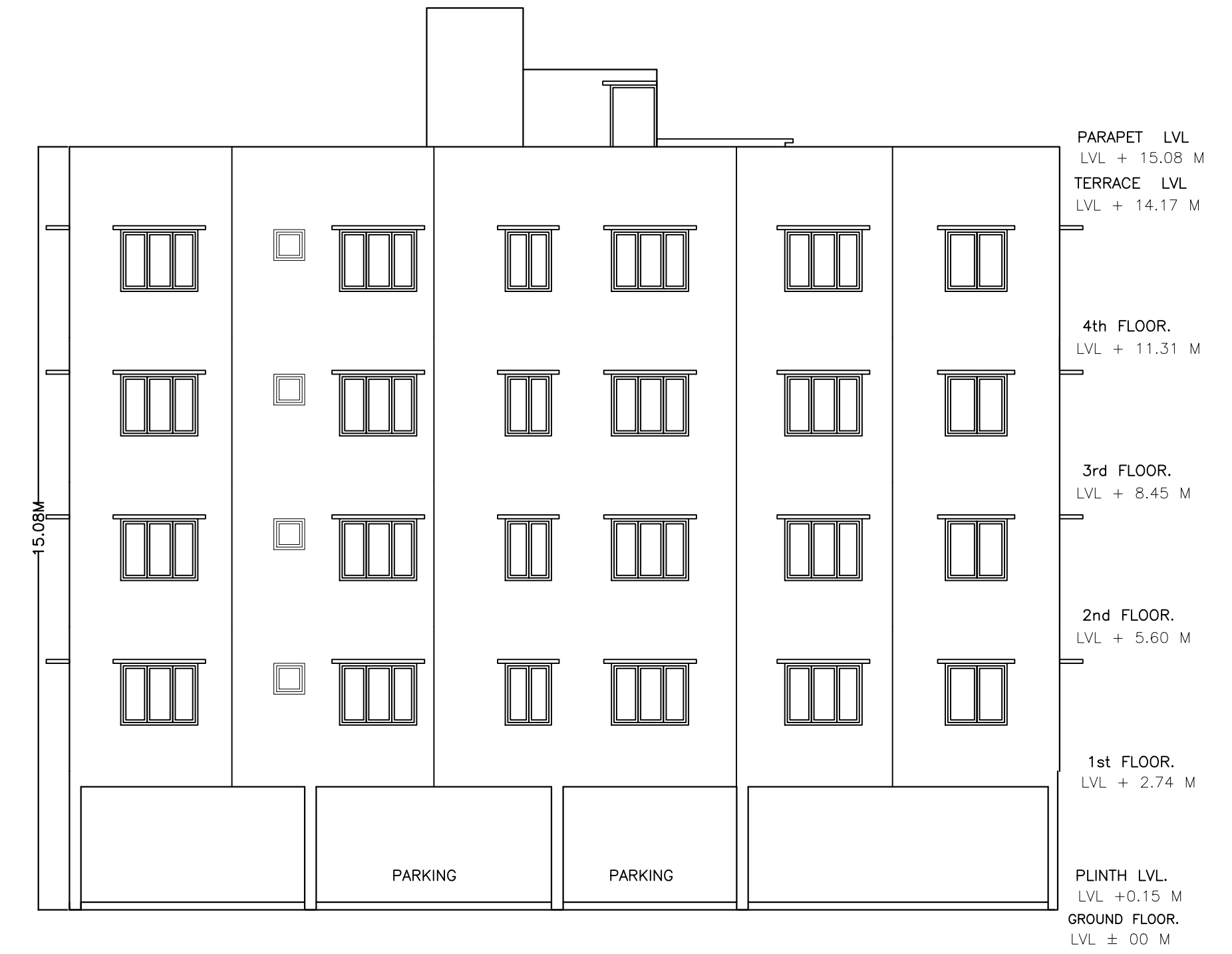
FRONT ELEVATION SCALE-1:100
