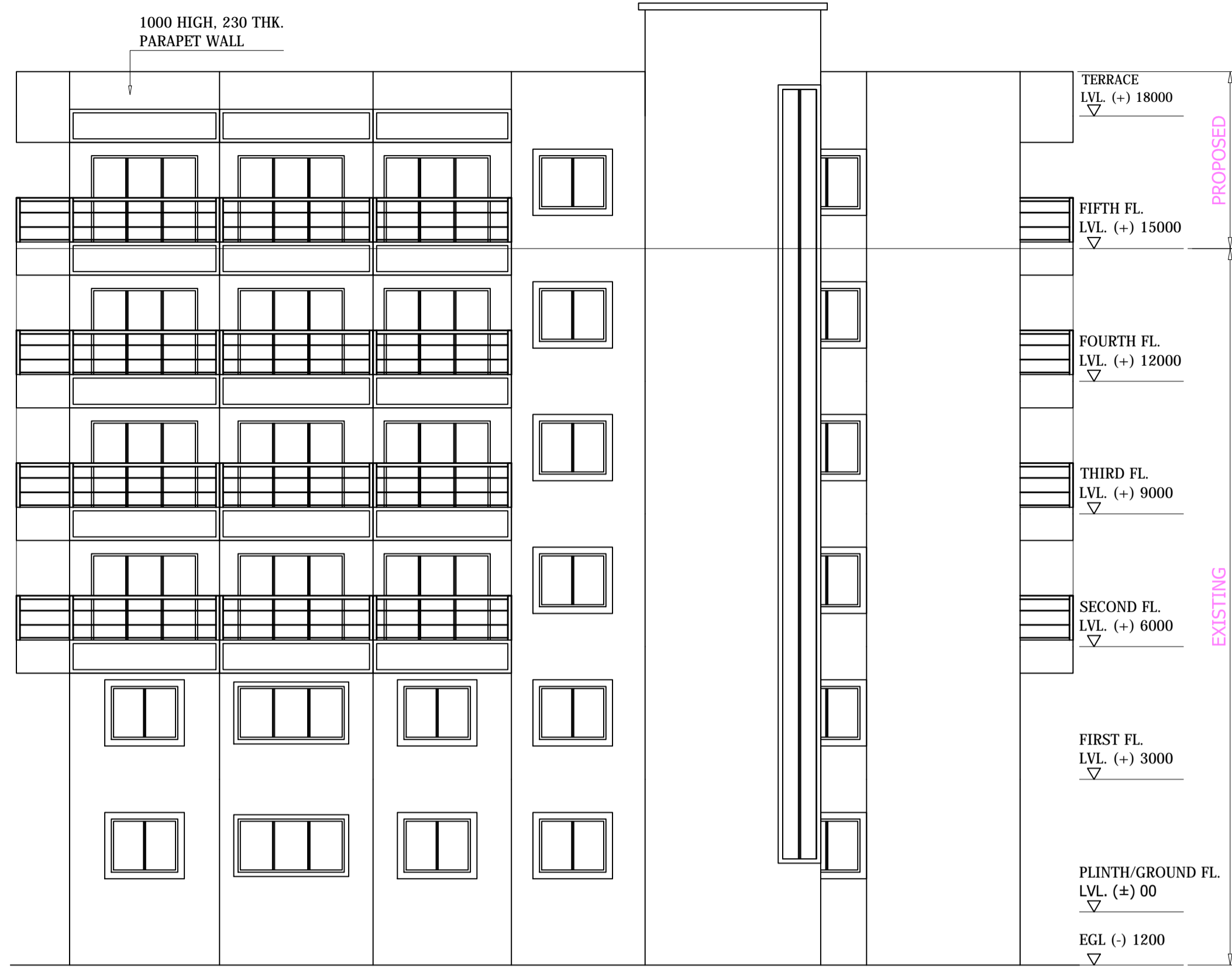
SOUTH SIDE ELEVATION - BLOCK A
