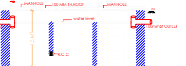
SECTION OF SEPTIC TANK
