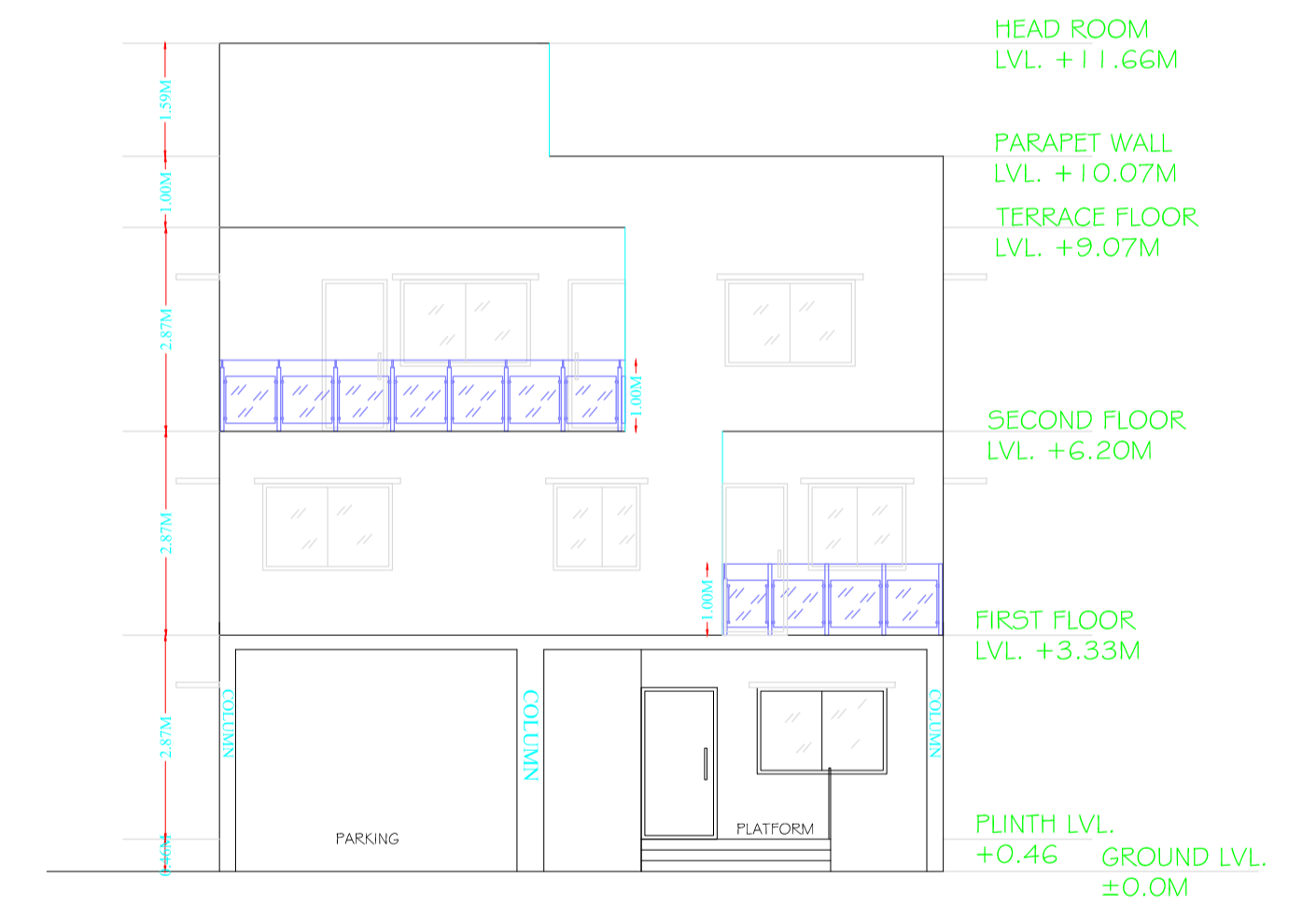
FRONT SIDE ELEVATION (NORTH SIDE)
