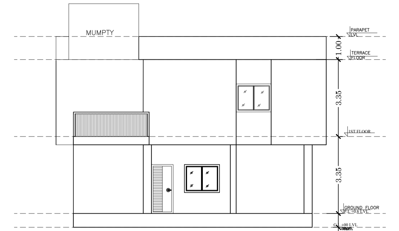
FRONT ELEVATION (SCALE 1:100)
