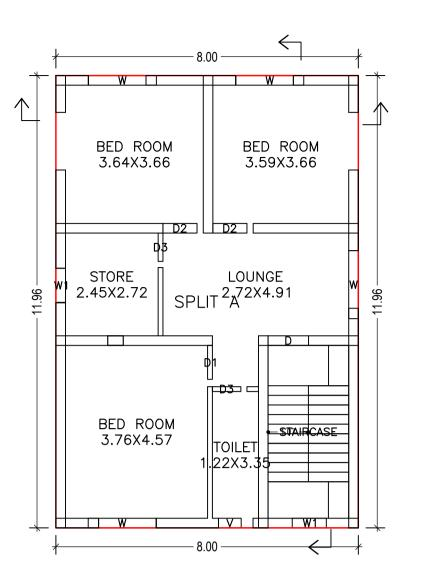
FIRST FLOOR PLAN (Proposed) (SCALE 1:100)
