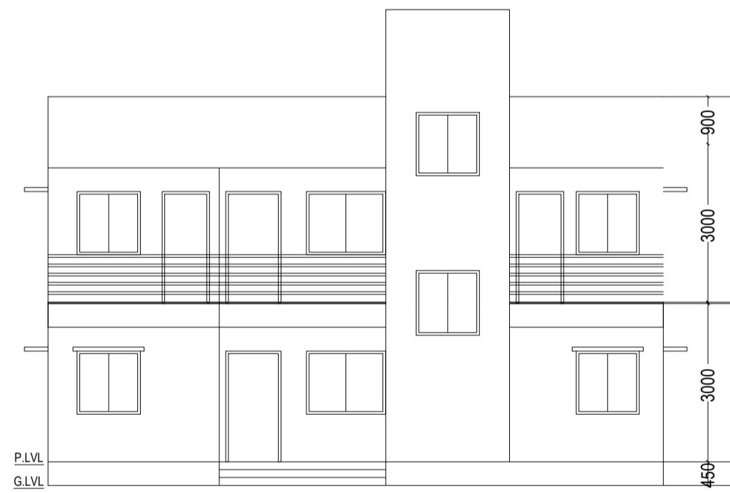
LEFT SIDE ELEVATION SCALE :- 1:100
