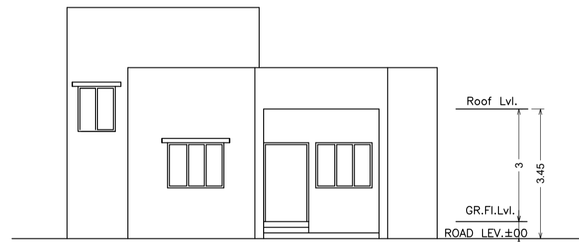
ELEVATION OF SIDE-A (SCALE=1:100)
