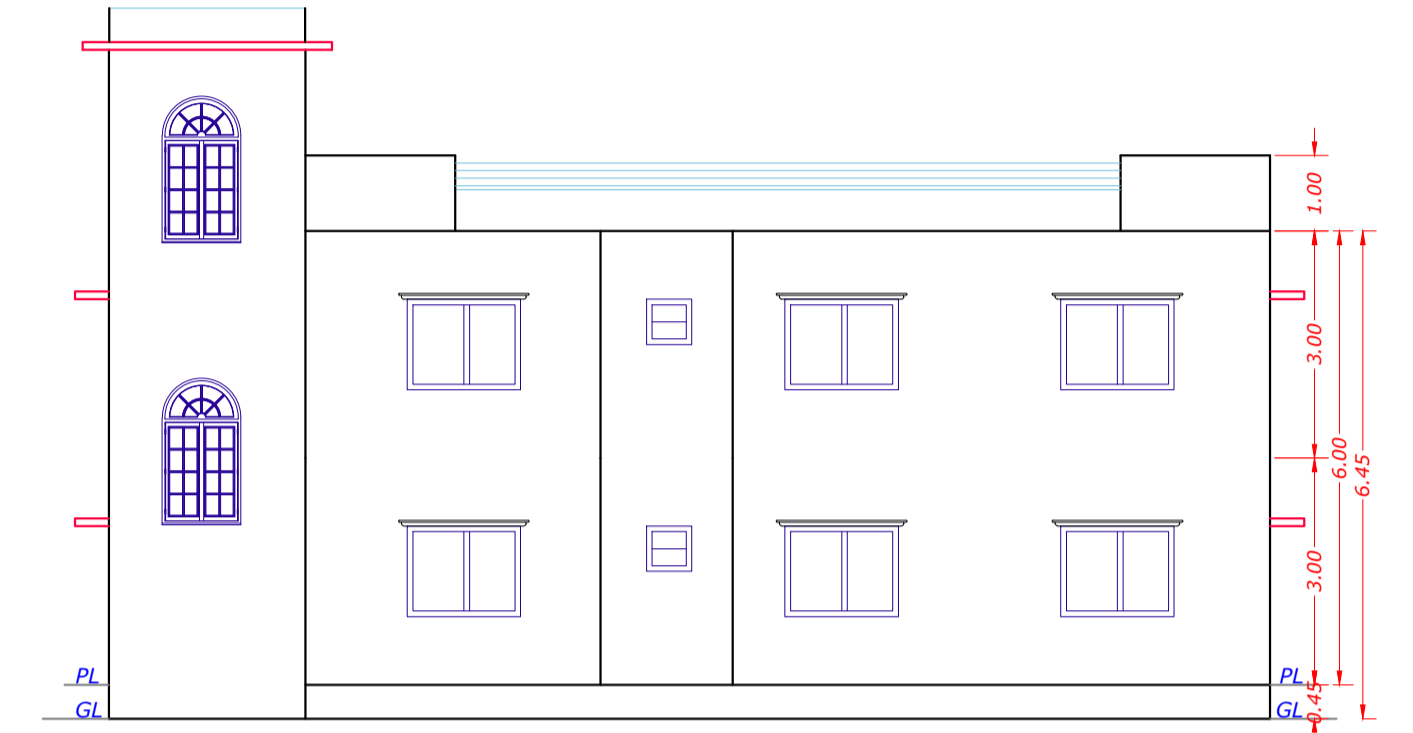
RIGHT SIDE ELEVATION (SCALE 1:100)
