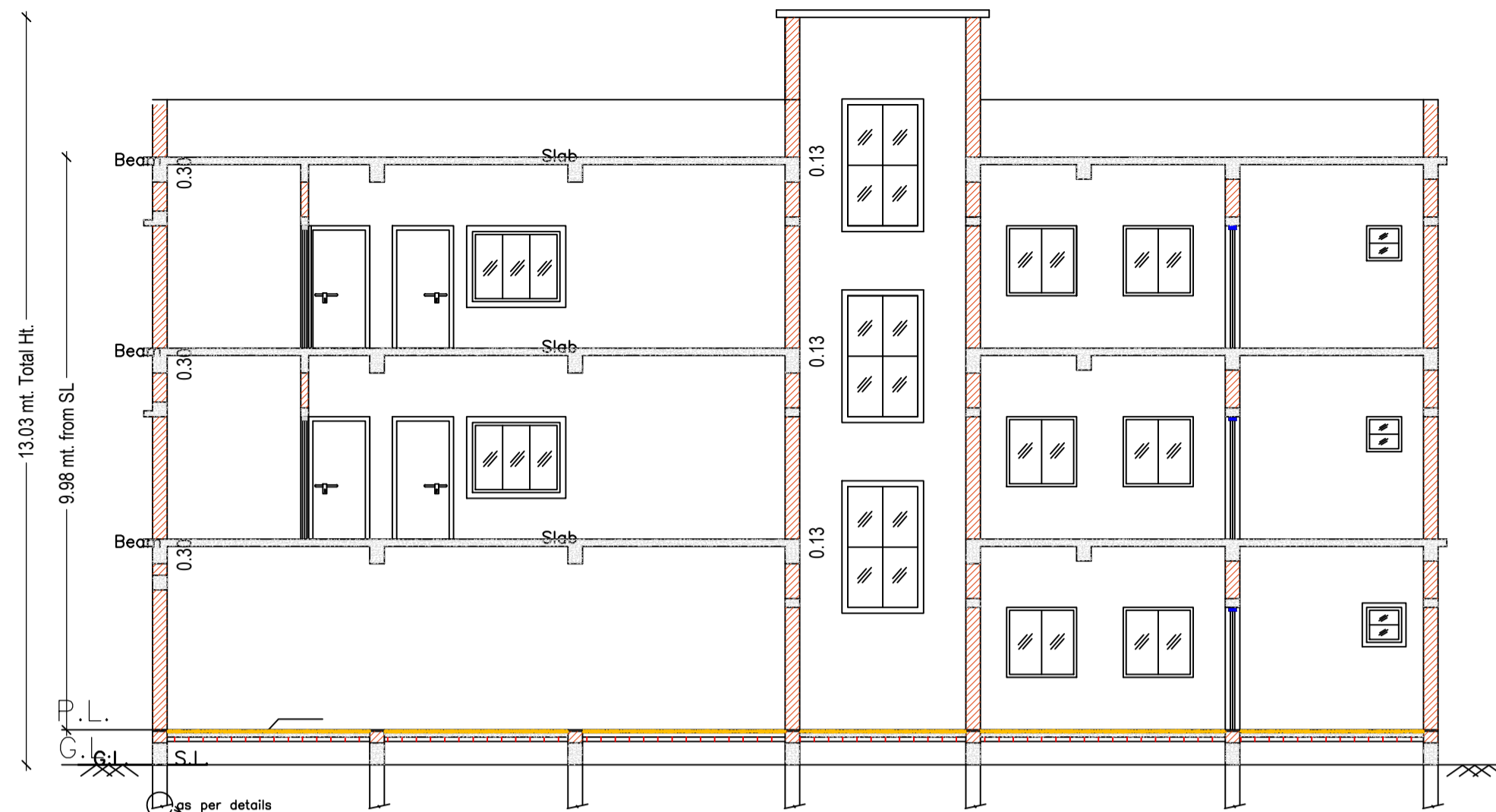
SECTIONAL ELEVATION AT Y-Y'
