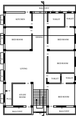
FIRST FLOOR PLAN SCALE: 1:100
