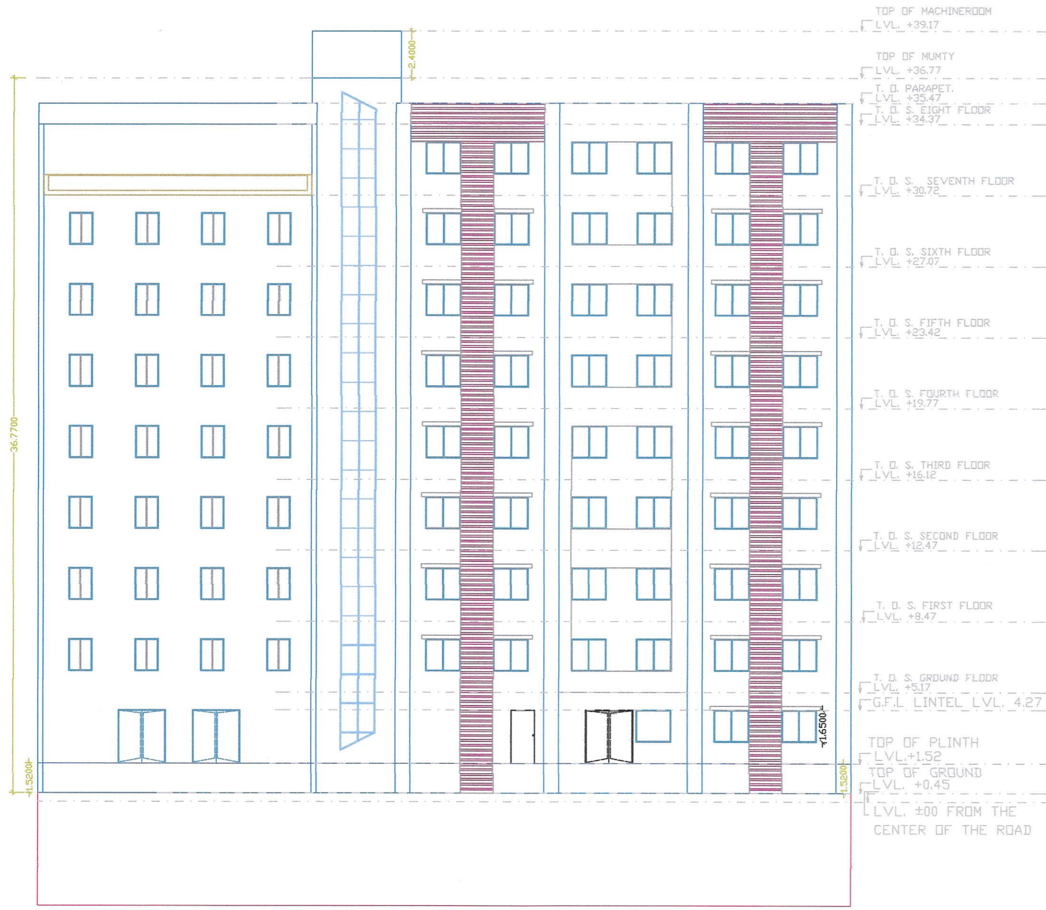
FRONT ELEVATION SCALE:1:100 NOTE: ALL DIMENSIONS ARE IN MTS. EXCEPT MENTIONED.
